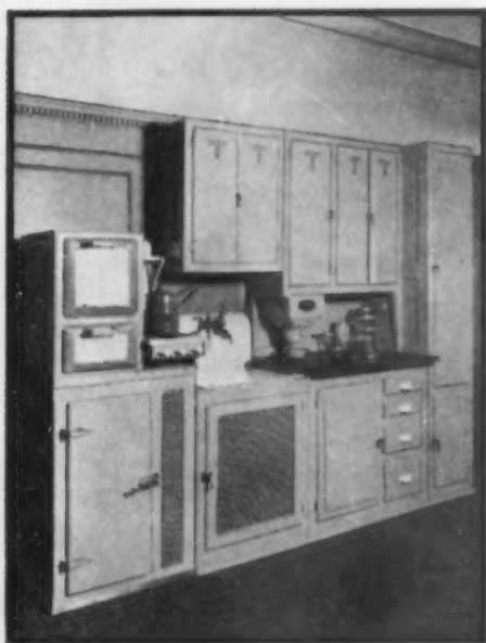
In this kitchen the gas range is installed in an alcove, with the sink, refrigerator, worktable, and cabinet conveniently arranged in relation to each other. (Photographs on this page courtesy Consolidated Gas Co.)
