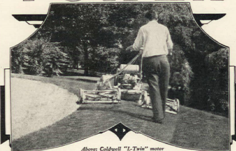
Above: Coldwell "L-Twin" motor lawn mower and roller. Mows and rolls simultaneously 4 to 6 acres a day. With Gang units attached it cuts a 60-inch swath, ten acres a day on one gallon of gasoline.
