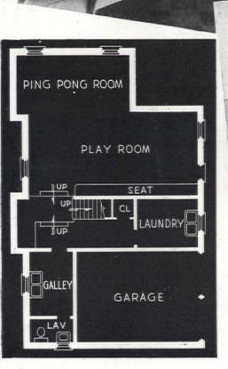
The cold closet is now a complete galley, equipped with an electric stove, sink, and cooking equipment. The far end of the original closet was partitioned off to make a lavatory
