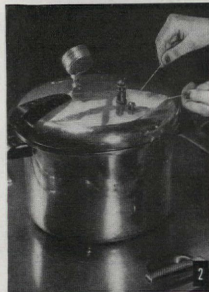
2. Clean pet cock and safety valve by drawing string or strip of narrow cloth through them
