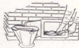
**B**elow the junction of the smoke pipe and chimney there should be an opening to provide access for cleaning dirt, soot, ash, and other loose material that collects in the base of the chimney. From this clean-out opening, you can shovel the sediment. When the cleaning is completed, the door or cover of the opening should be fitted or sealed to eliminate leaks that were detected with the lighted candle. If there's no clean-out opening, remove the dirt through the smoke-pipe opening.
