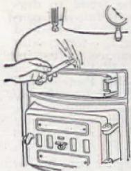
With the fire burning, a lighted candle will indicate leaks as the flame is drawn into or toward the boiler. Leaks may be around any doors, dampers, covers, joints in the smoke pipe or by the chimney, and miscellaneous cracks. On some heating equipment the jacket must be removed before all leaks can be found. These leaks cause inefficient burning of the fuel and loss of heat up the chimney.
