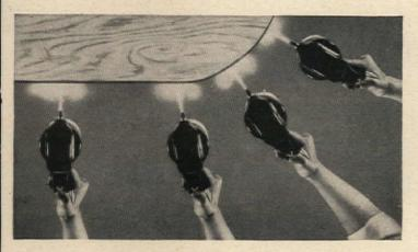
Bird's-eye view from above. With both flat and curved surfaces, keep the spray axis at right angles to the point of impact, keep the gun horizontal and an even distance from the surface, and move it at a uniform speed to desposit an even spray, without floods or misses. The distance and speed of moving the gun varies with the paint texture and the spray-gun tip. Experiment a bit before doing each job
