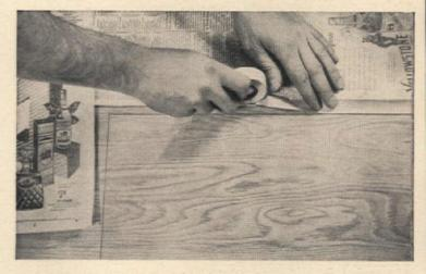
With pencil line or other indication, mark off area to be sprayed. Cover adjacent areas with newspaper to keep them from being sprayed, too. Masking tape holds paper in place and enables you to achieve a clean, sharp edge for the sprayed area. Smooth the tape down firmly over the pencil mark to make sure that none of the paint creeps under the mask to make the edge ragged and messy
