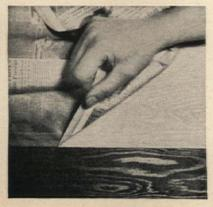
Usually at least two or three coats are needed. When the last coat is completely dry, pull the tape away at a sharp angle, doubled back on the mask to insure a clean edge. Tape will break away and not pull off the newly sprayed area
