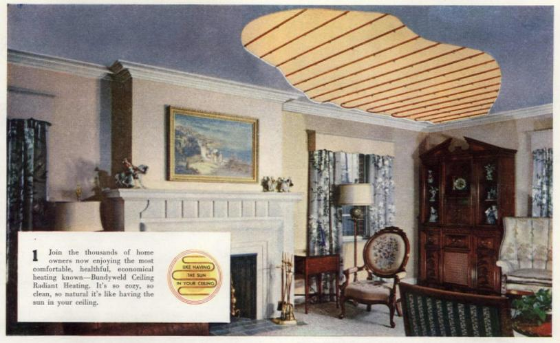
Today's big news in home comfort is made possible by the fact that radiant rays will travel downward. Cutaway view shows coils of Bundyweld Tubing hidden in plaster ceiling.
