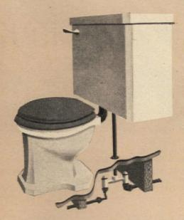
Condensation on the outside of flush tanks can be cured by bringing warm water into the tank. A special fitting is used to connect a hot-water line to the cold-water supply to the tank
