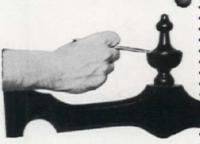
To sand intricate carvings or moldings, fold a strip of fine sandpaper over the end of a stick sharpened to a chisellike edge. Hold stick like a pencil and work it along the surface. Shift paper to clean grit if it becomes clogged
