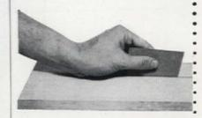
Try this next time you edge, join, and glue two boards. Slip a piece of folded abrasive paper or cloth between the two edges and sand off high spots that prevent the boards from meeting evenly
