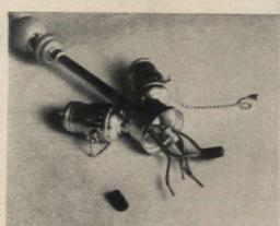
Tuck wires into the head of lamp so that solderless connectors face each other; keep twists and criss-crossing down to minimum. Don't replace head of the lamp till plug end of cord is rewired.
