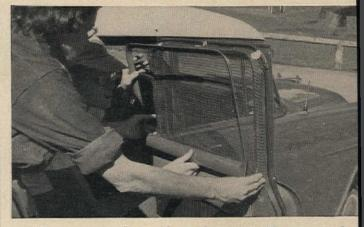
Unscrew car window molding and remove it. Then tape in place "screen"—a panel of net that's 6" wider and longer than windo
