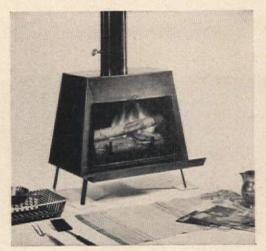
This lightweight, prefabricated metal fireplace is low-cost. It burns coal, charcoal, briquettes, logs up to 18". Its stovepipe can be installed directly through roof of your vacation house, using ordinary sheet-metal roof flange, flashing.
