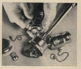
First disconnect plug from wall outlet. Remove top of lamp where separate wires are joined. Then separate shell of sockets from the socket caps, as shown: you press in sides of the shell and pry with screwdriver.
