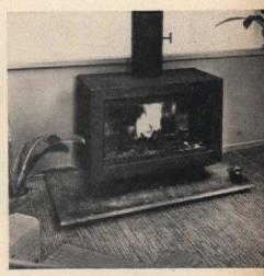
Simple in design, this steel fireplace has 3" space between inner and outer walls. Pulls in cool air at bottom, heats it around firebox, then sends it out warm.
