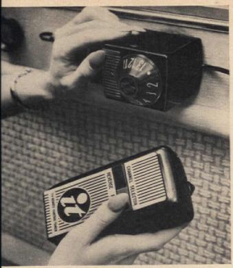
REMOTE-CONTROL TV TUNER can be attached to front of standard television set for changing channels from any place in the room. It fits without electrical connections, operates on flashlight patteries. Priced at \$19.95. Alliance Mfg. Co., Alliance, Ohio.
