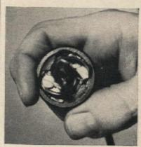
Tie a knot in the cord where it comes through base of lamp. This reduces the amount of inner play that might cause damage to insulation, and eventually a crossing of "hot" wires and trouble.
