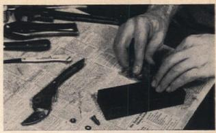
It's easy to take pruners apart and sharpen them on an oil stone Sharpen blade of an anvil-type pruner on both sides, as a knife; blades of a scissor-type shear only on beveled side; stone other side flat, gently, to remove wire edge or burr.
