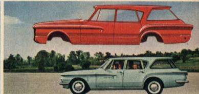
**More room, less noise.** Solid welded Unibody ends the major cause of squeaks and rattles, adds inches of space inside by getting rid of bulky body-on-top-of-frame construction.
