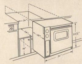
Stack-on ovens, sometimes called "modular units," save installation expense. They need no special enclosure as top and sides are finished, and they may be installed flush to the wall. The compact cluster surface cooking top, a popular space saver, has separate control panel below. (See details at left.)
