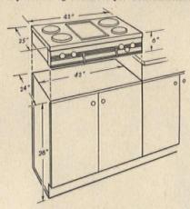
Fold-down surface cooking tops qualify as stack-ons because they need no cut-out; ideal if counter space is shy. Attached at rear, they project less than 6" when closed, Gas or electric.
