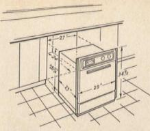
Under-counter oven has front panel same height as standard base cabinets, slips into space 27" wide. Levelers in base adjust height according to thickness of counter, assure snug fit. Front panel trim overlaps cabinets on each side. Oven is designed to allow space for a drop-in surface cooking top in counter above, if you want to combine cooking and baking areas. A regular built-in oven would need some kind of base support for installation below a counter.
