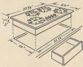
Drawer will fit under any surface cooking top that is not over 3" deep. Like built-in ovens, drop-in tops always extend slightly over edge of counter cutout to form a tight seal. Some lift up for cleaning.
