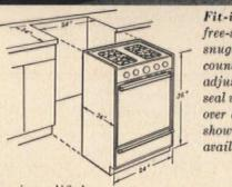
Drop-in range is modified built-in. Fits between base cabinets, into U-shaped cut-out. Costs less to install than separate built-ins.
