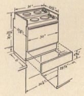
This fit-in range (above and below) looks like a drop-in, but stands on the floor with counter at sides and back.
