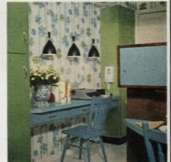
The 30" high counter at the end of the island work area is a perfect mixing height. Mixing equipment and nonrefrigerated vegetable storage are below. An electric outlet at the back of the counter allows you to use small appliances on the spot. Midway units hold an extra supply of spices and small utensils.
