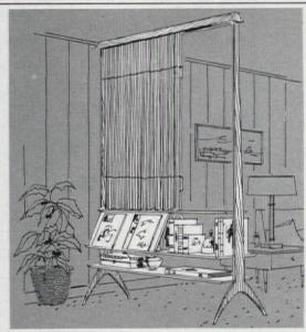
A slatted wood curtain, hung on a track inside the wood cap, provides any degree of opening desired. Below it racks and shelves are fastened between the uprights.
