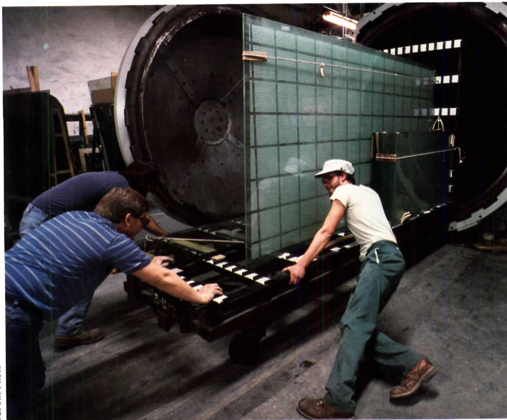
Left, laminated safety glass is removed from autoclave. Facing page, from top: silicone sealants attach glass dome; PVB safety-glass sheeting; and heat mirror glass production.
