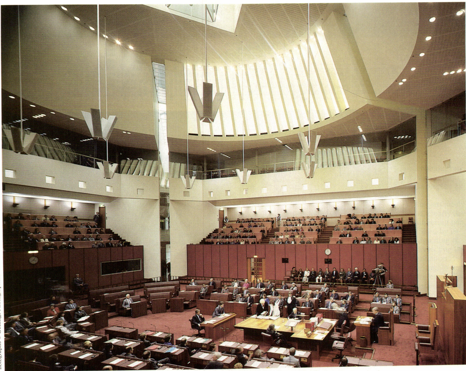
Above, the Senate chamber lighted by clerestory slots in elliptical drum; eight speaker clusters are suspended from ceiling. Facing page, clockwise from top: the members' hall with screen wall supporting pyramidal skylight over square reflecting pool; the hypostyle foyer with columns partially clad in marble and strong floor patterns; and the square-plan House of Representatives chamber with lights on suspended track.
