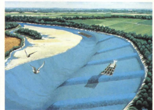
BENDWAY WEIRS: Stone structures harness Mississippi.
