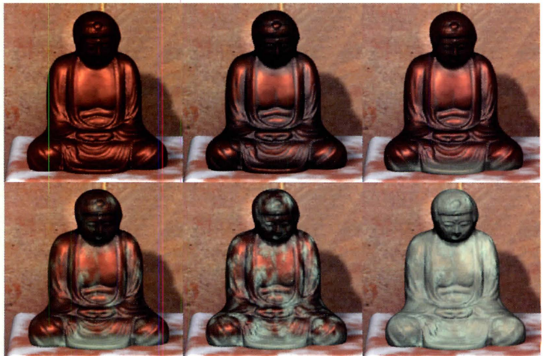
Computer model of copper Buddha simulates tarnishing and development of patina over time
