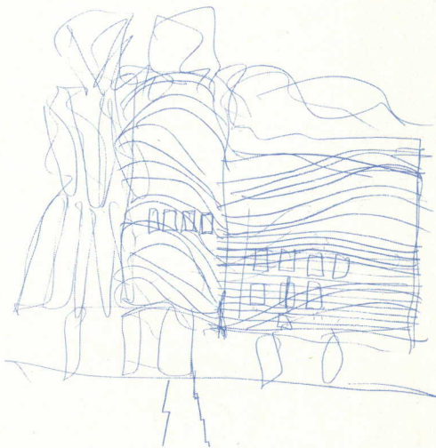
Conceptual sketch by Gehry shows waves in facade, which mediate between his towers' verticality and the surrounding block's dominant horizontality.
