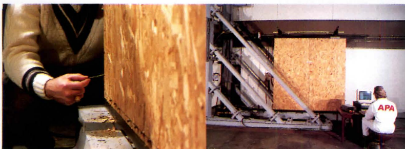
APA researchers test the seismic performance of a plywood shear wall.
