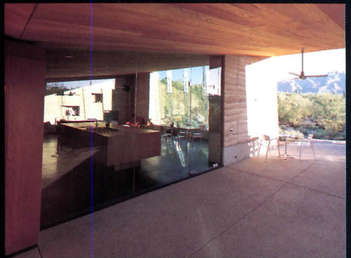
Fireplace in massive rammed-earth pier warms porch (above) during winter. Pivoting glass door (right) connects kitchen with porch.
