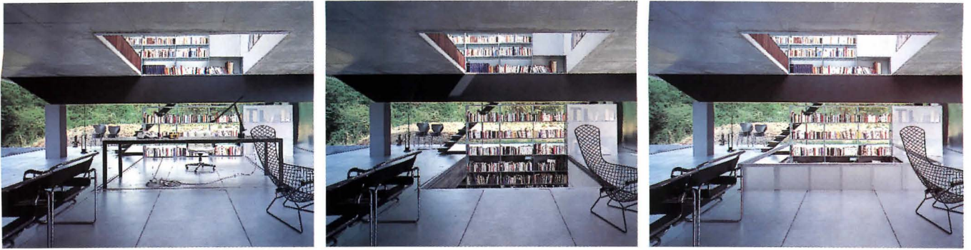
In sequence of photos (above), descending elevator opens view of multistory library. Low peripheral walls surround void for safety of ambulatory residents.
