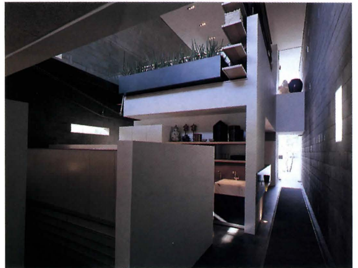
View from principal's office to open conference area reveals narrowness and permeability of single-loaded volume (above right). Wooden planks of bookshelves conceal steel columns supporting conference-room floor, a trick Burnette borrowed from Frank Lloyd Wright. Interiors soar from small entry lobby (below left) to double-height work area at rear (below right). Glazed facades at studio's front and back create fluid, luminous interior.
