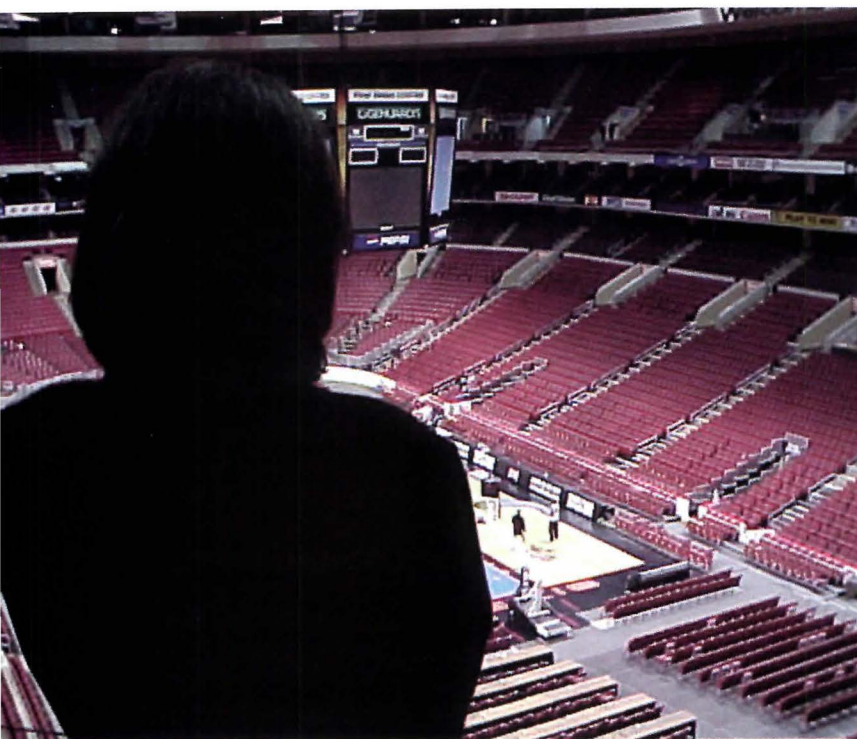
Photograph used by disabled advocates in lawsuit to demonstrate obstructed sight lines at Ellerbe Becket's First Union Center in Philadelphia. Advocates charged architects with hiding wheelchair seating beneath three removable rows of seats, so that as many as 48 seats had to be folded up to accommodate disabled customers.
