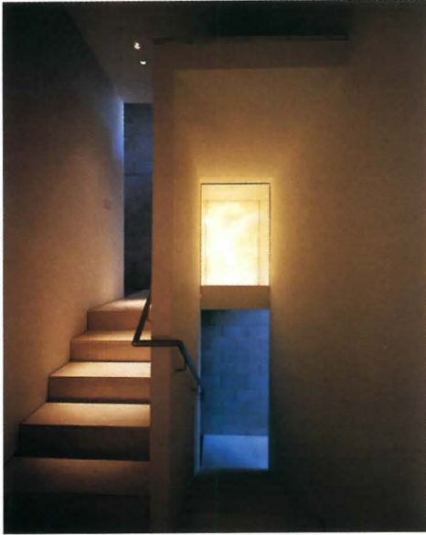
Onyx panel set in masonry wall casts moody glow in staircase. Daylight from glazed vitrine falls on stair landing.
