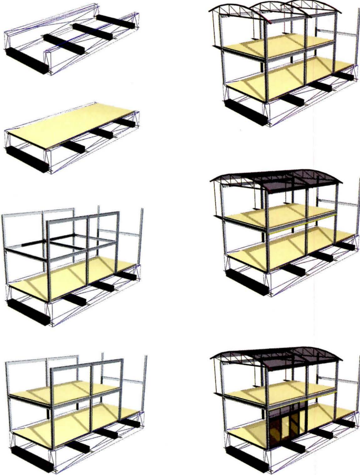
House_n innovations include development of factory-produced building components (above), shown here as sequence of diagrams by MIT students Ryan Chin and Louie Tak Wing. Other student participants are Abir Ahmad, Katherine Calef, Gregory Demchak, Lucy Fang, Laurie Griffith, Sini Kamppari, Lee Knight, Christopher Mulvey, Junko Nakagawa, Kevin Settlemyre, and Michael Wilcox.
