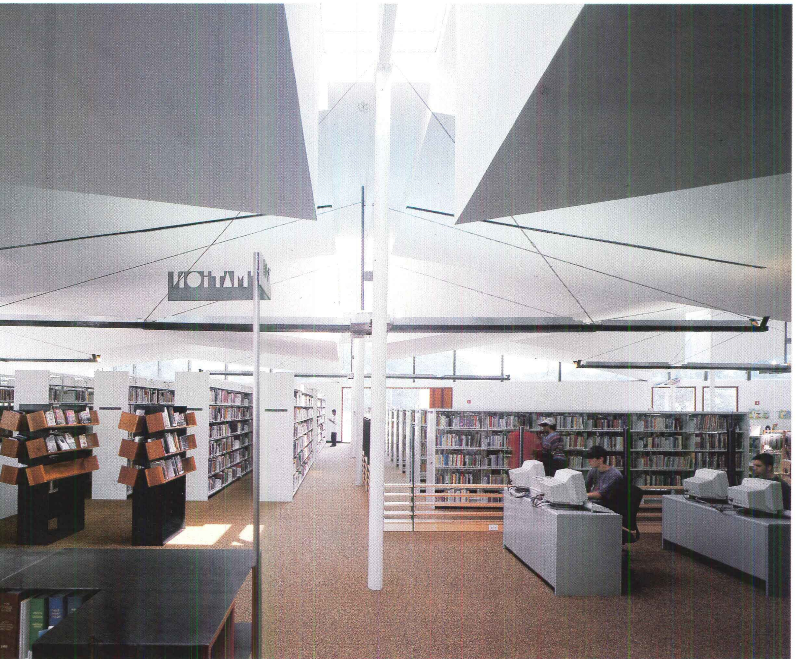
Full-height windows at floor level illuminate reading areas on the perimeter of the library (above). Light from skylights and the triangular clerestory windows washes across the ceiling (facing page).
