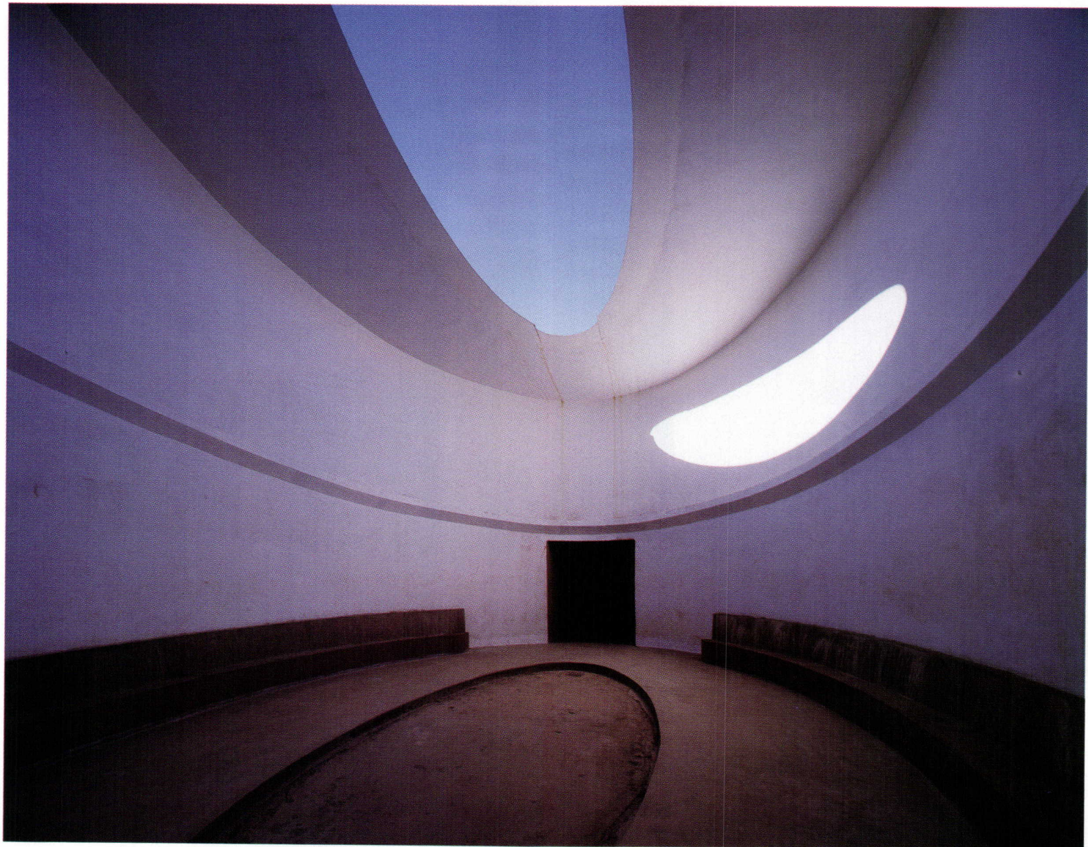
3 Turrell installed rosa sandstone–faced pews around the long sides of the elliptical East Portal Space (facing page) where visitors can view the sky through the oculus above. The oval recess in the floor will be filled with white silica sand, filtering rainwater into a drain. A low, curving passage (above, at rear) leads to the only orthogonal space in the crater (below), a sort of antechamber to the crater's eye.
