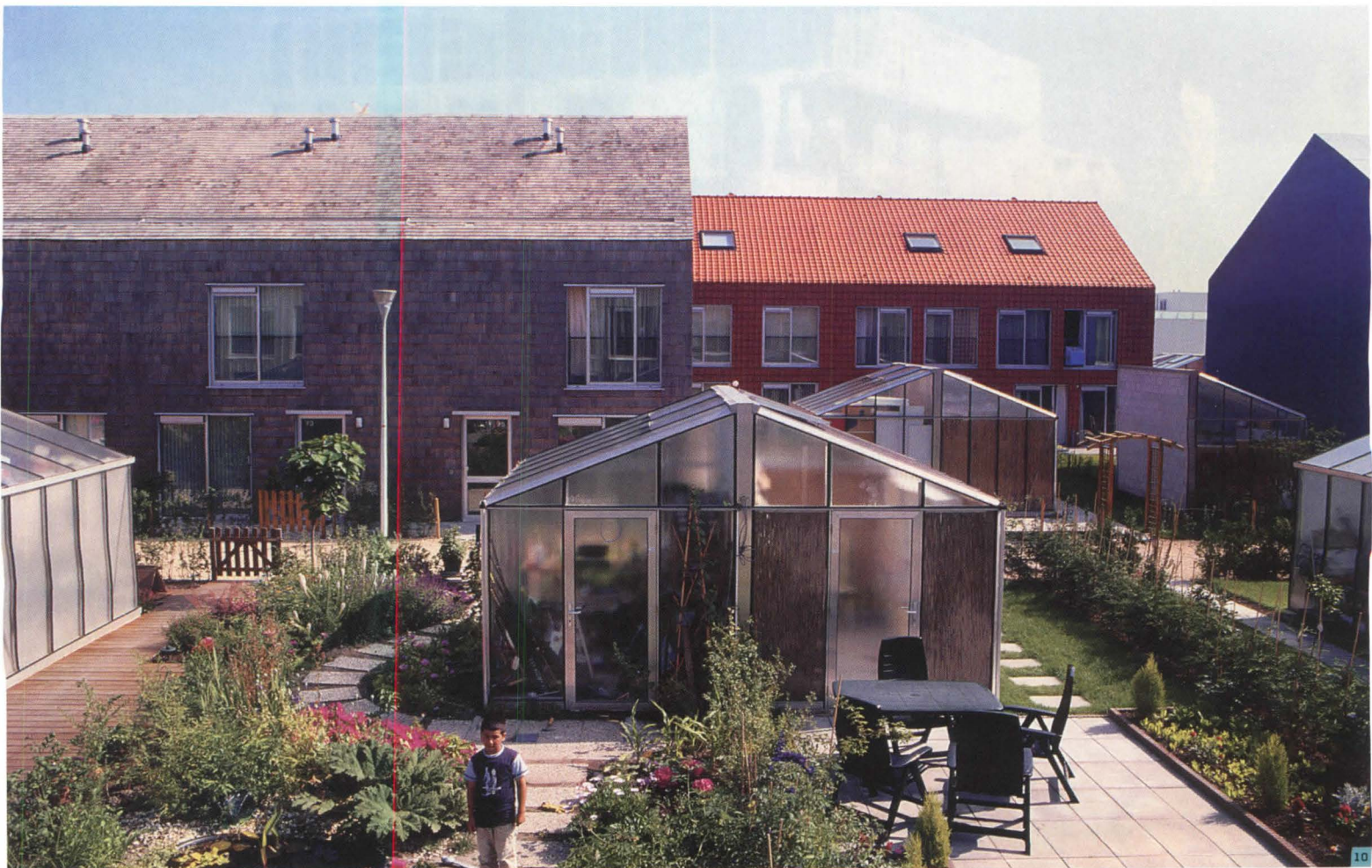
At Hagen Island, a 119-unit, moderate-income housing development built on former marshland, the architects make the generic unique with skins that start at the peak of the roof and end where the house meets ground (8). Though the details the firm developed to allow it to use roofing materials like clay tiles (10) as siding have performed well, there have been problems with water seepage around doorbells and windowsills. Hedges and fences (9) have been added in defiance of residency guidelines.
