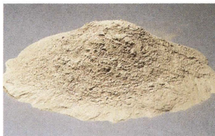
Fly ash is captured from the exhaust gases of burning coal.
