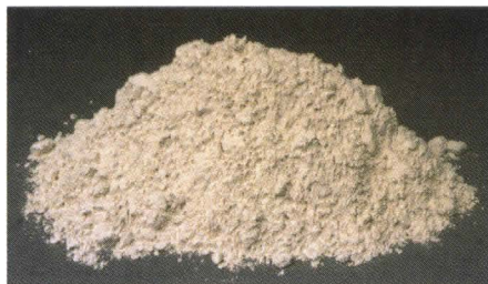
Slag cement is a reclaimed, recyclable industrial by-product of the iron- and steel-making process.
