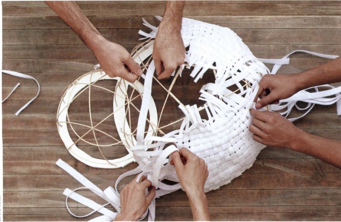
The final model for Ukendt/Igloo served as a template for how its felt surface would be woven into the structural frame.
