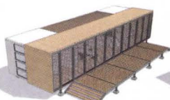
Stairs are dropped to existing grade level
