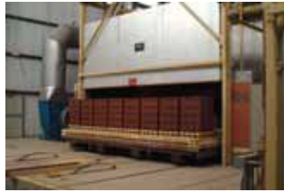
Figure 4. Brick exiting tunnel kiln
