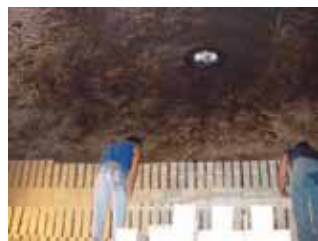
Figure 5. Brick being stacked in beehive kiln
