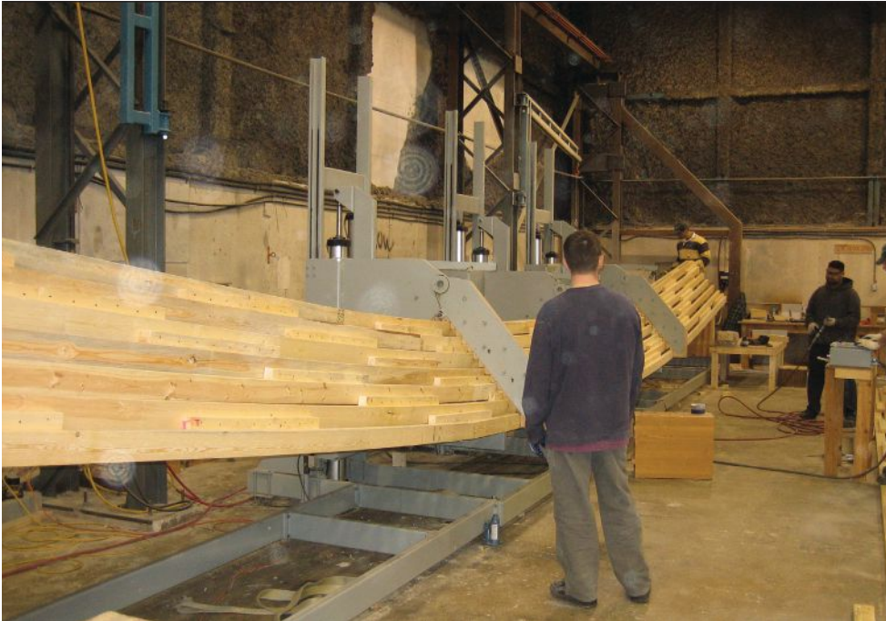
The one-of-a-kind Richmond Oval roof structure is comprised of dimensional lumber and Douglas-fir plywood fabricated into WoodWave panels and also includes Douglas-fir glulam beams. Architect: Cannon Design. Engineer: Fast+Epp Structural Engineers. Photo credit: www.naturallywood.com
