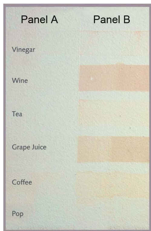
These paint test panels have been exposed to common stain agents found in restaurants and retail stores. Panel A was painted with a high quality latex formulated with excellent stain resistance and washability, while Panel B was painted with a standard latex. Panel A wipes clean with water and mild detergent, while Panel B is permanently stained.
