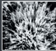
Xypex Crystallization (Mature)
