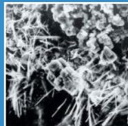
Xypex Crystallization (Initiated)
