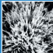
Xypex Crystallization (Mature)
