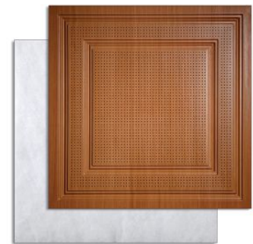
Noise reduction as high as 0.85 NRC is available with perforated thermoformed ceiling panels in combination with a thermal-bonded, polyester fiber, non-woven batt. Panels and batts are Class A rated for surface burning characteristics and panels are Greenguard Gold certified for low VOC emissions. The faux wood finish shown here provides verisimilitude when viewed at normal ceiling heights. Photo: Ceilume
