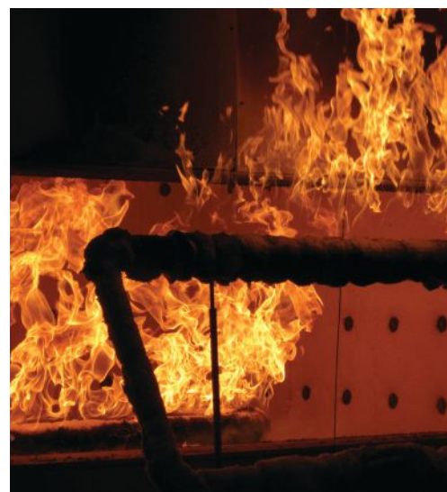
The International Building Code requires that walls with foam plastic insulation pass the NFPA 285 test. Image courtesy of Construction and Maintenance Solutions, LLC
