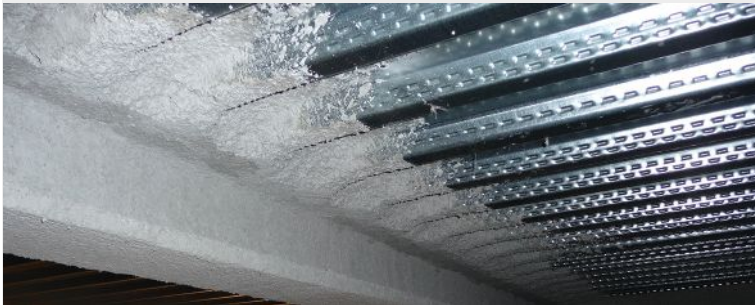
An unrestrained, steel-framed floor specimen before and after a fire test. Photo courtesy AISC
