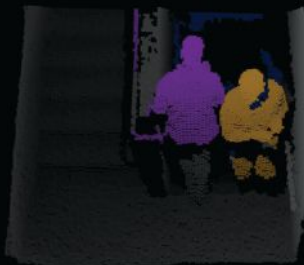
Infrared cameras track user speed, direction, peak use times, and collision rates on stairs in ZGF's Seattle office.
