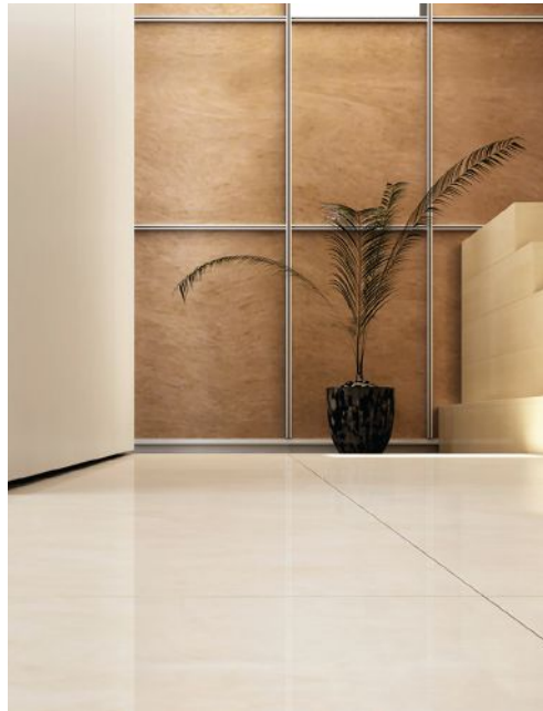
Extruded aluminum can be used to create minimalistic reveals with drywall (left wall) or bold accents with other panels (rear wall)
