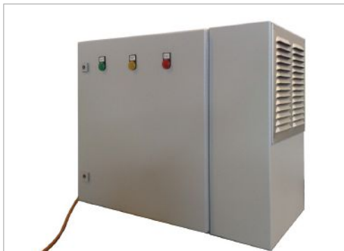
The air supply units inflate the cushions and are equipped with two fans: one for standard operation and one for backup. They can easily be fitted with dehumidifiers, which is recommended for high humidity environments. The air supply unit cycles to provide air for the cushions as needed. (Image © Vector Foiltec)
