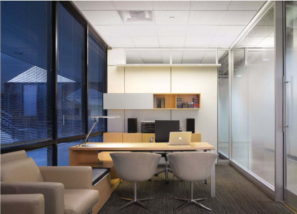
To preserve flexibility, walls are often built to the suspended ceiling or using demountable partitions. Walls may include substantial windows or even be built in glass from floor to ceiling. CREDIT: Benny Chan/Fotoworks
