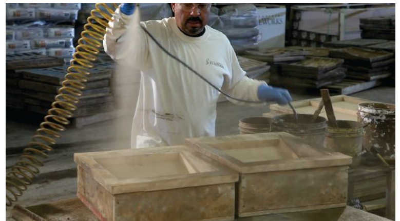
Figure 2. Manufacturing and applying color to molds in the Denver, CO manufacturing facility.
