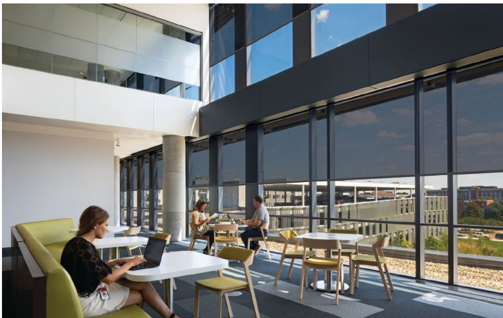
Shades are a critical component for managing daylight and preventing glare. Photo Credit: Photo © Chris Cooper
