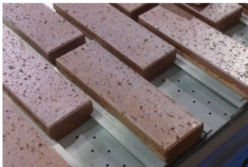
Bricks are permanently secured into custom perforated trays.
