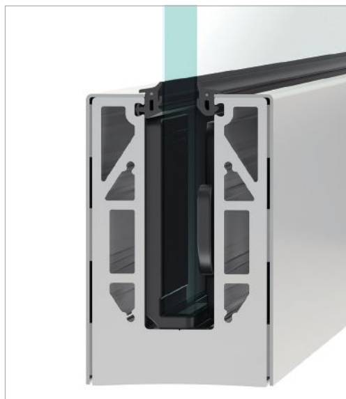
Some base shoes feature a multiple-hollow design that makes them 30% lighter.
