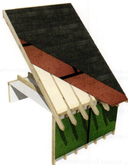
Unvented roofs with conditioned attic spaces place the air, vapor and thermal control layers near the roof sheathing.
