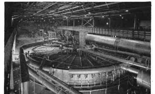
The world's largest Rotary Billet-Heating Furnace in our No. 3 Seamless Tube Mill, Indiana Harbor Plant.
