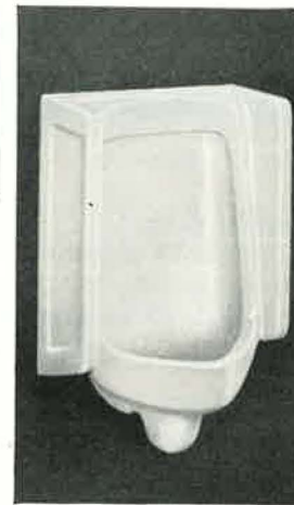
Briggs Lawton Urinal specified for Bissell's new plant displays cleanly sculptured design. All 14 are wash-out, include integral extended shields, flushing rims, integral china strainers and trap with cleanout. Six colors and white.
