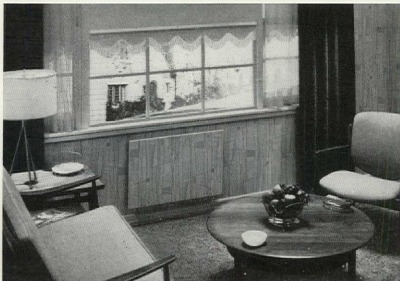
INSIDE , the new Thinline air conditioner panel can be painted or papered to blend in with room décor. Easy-to-reach controls are hidden from view.
