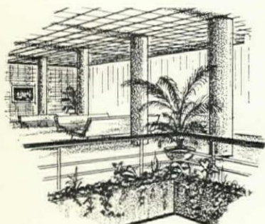
Used in, or adjacent to glass walls, round columns offer minimum obstruction to light and occupy minimum space.
