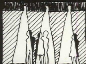
BC—change from narrow-beam spots creating dark and light floor patterns.
