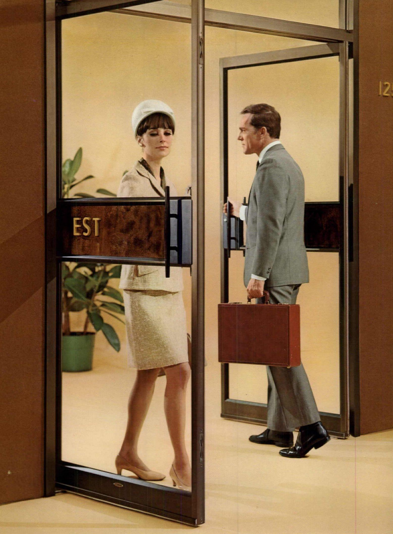
STYLE LEADER 125 ENTRANCE. Unlimited options in center identification panel, using any quarter-inch thickness material... wood, porcelain, plastic, glass. Permits customizing of standard doors. Each 125 has weathering on all 4 sides. Top and bottom locking bolt eliminates cut-out in door stile. Closer concealed in transom.
