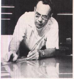
The stainless sheets marked up here for press vork, were formed by the mechanical conractor, Temp-Control Corp., Portland.
