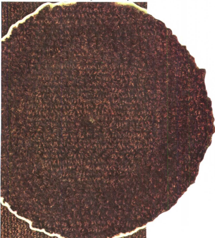
Acrylic after 1,800 cycles on a Taber Abrader. Fortrel PCP after 1,800 cycles on a Taber Abrader.
