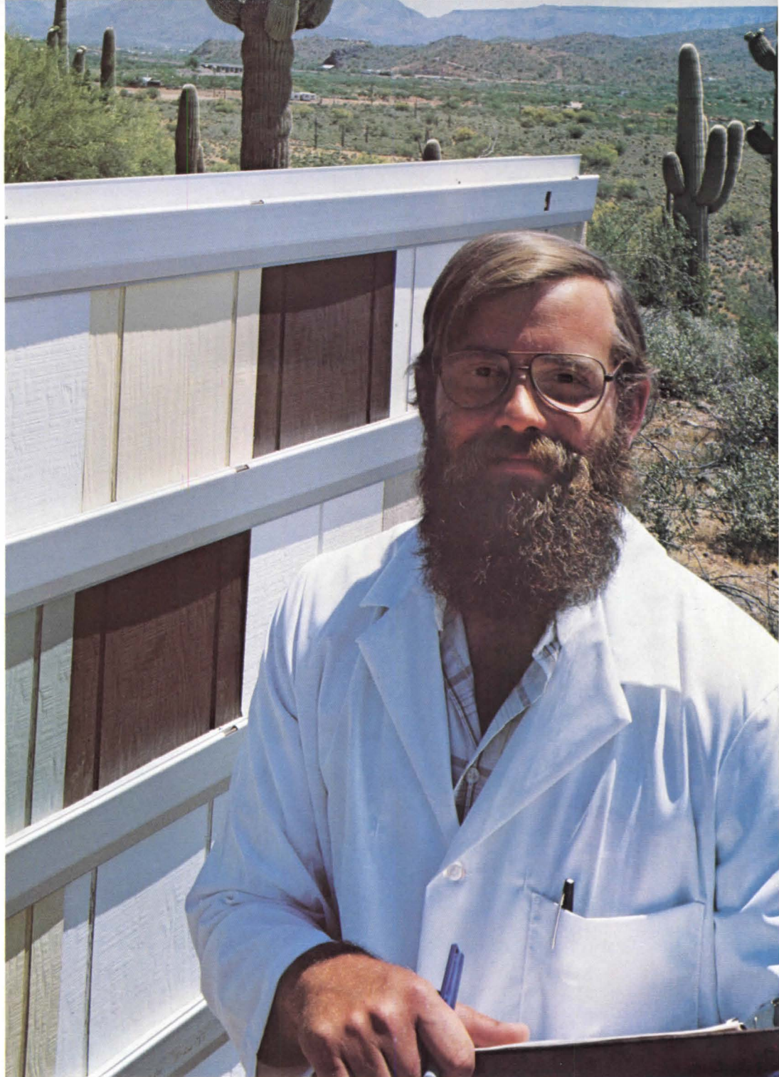
Ruf-Sawn 316 after seven years of exposure
