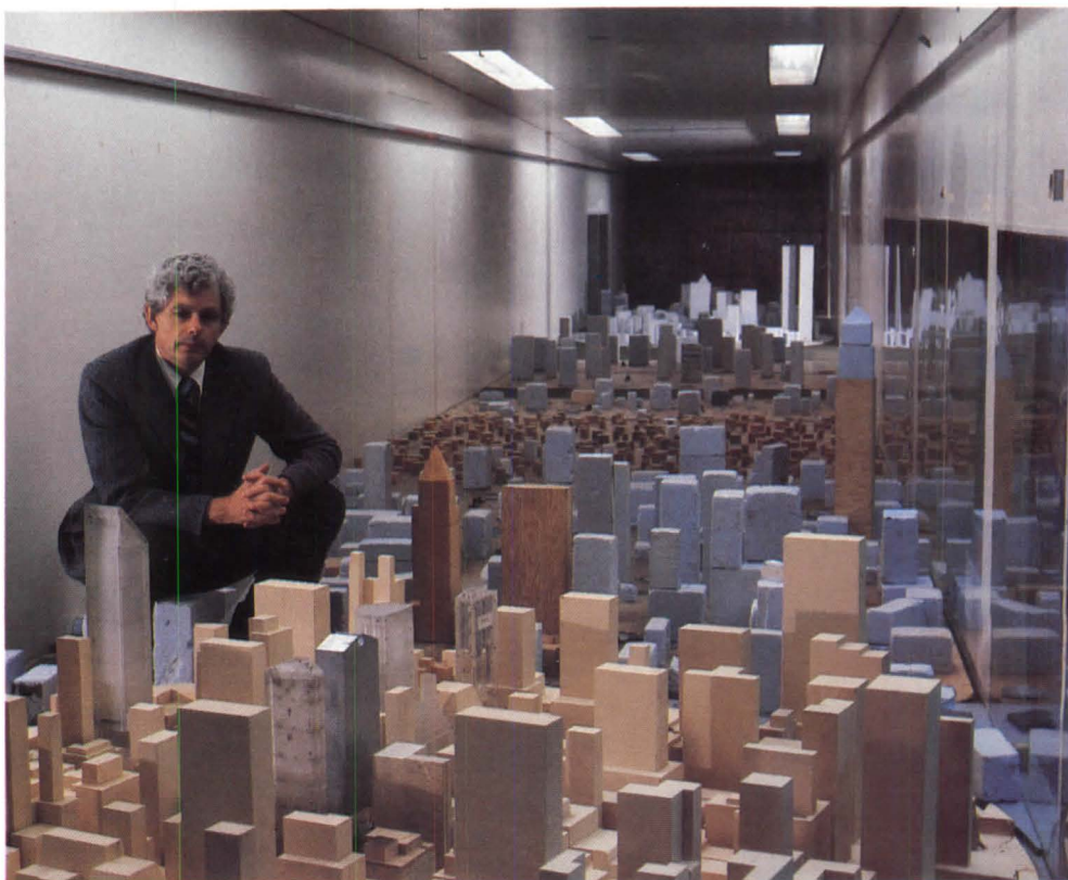
Model structures for testing in a wind tunnel.
